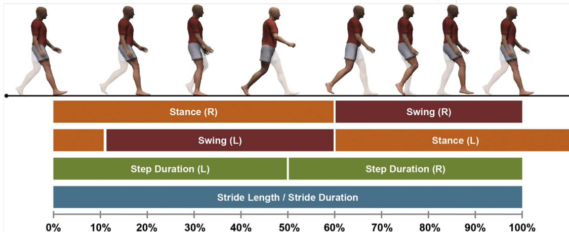
Fig. 1. Schematic of the human gait cycle and the spatiotemporal parameters validated in this study. Specifically, we validated the IMU system's ability to measure the stance percent, swing percent, stride duration (gait cycle time), stride length, and step duration in addition to the speed and cadence of the cycle.
